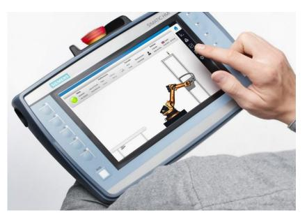
Featuring a 16:9 aspect ratio and 16 million colours, the brilliant widescreen display provides clear, detail-rich visualisations, even of complex process and plant images, such as the Vertical Lifts.
